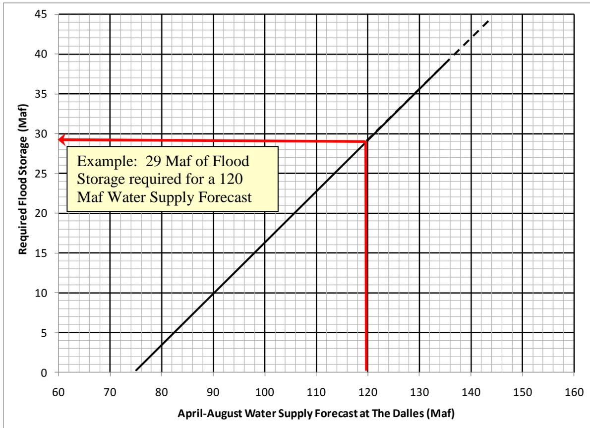
**Figure 2 - Chart for Determining Flood Storage Requirement (Proposed)**
