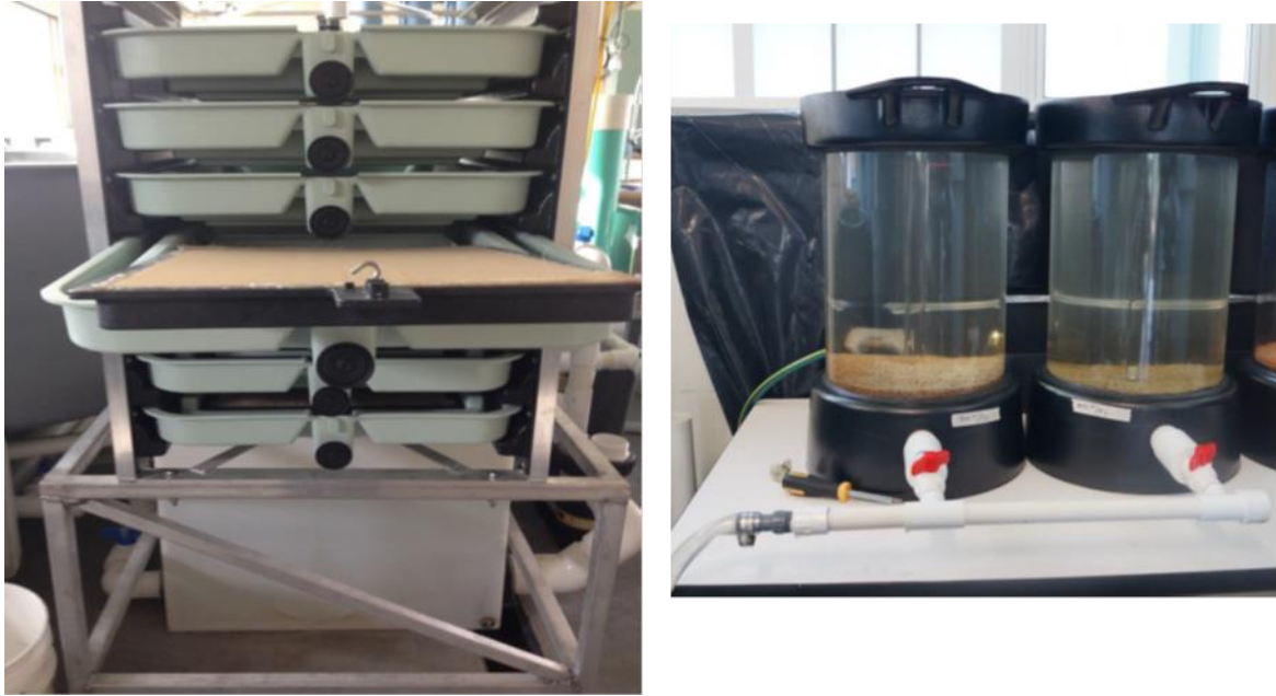
Figure 5-11. Heath rack (left) and Eager upwelling jars (right) modified for lamprey egg incubation.
