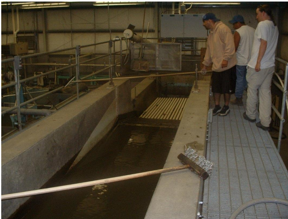
Figure 5. Inside view of the Chandler Evaluation Facility showing the separator rack where kelt steelhead are collected.
